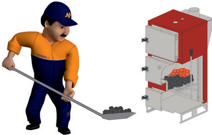
Figure-16: Load sufficient enough crude coal to the empty place on the front of the grate.
