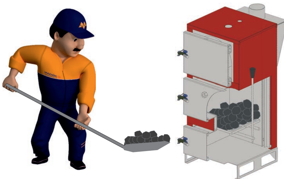
Figure-12: Load until the fuel height is 10-15 cm on the grate.
