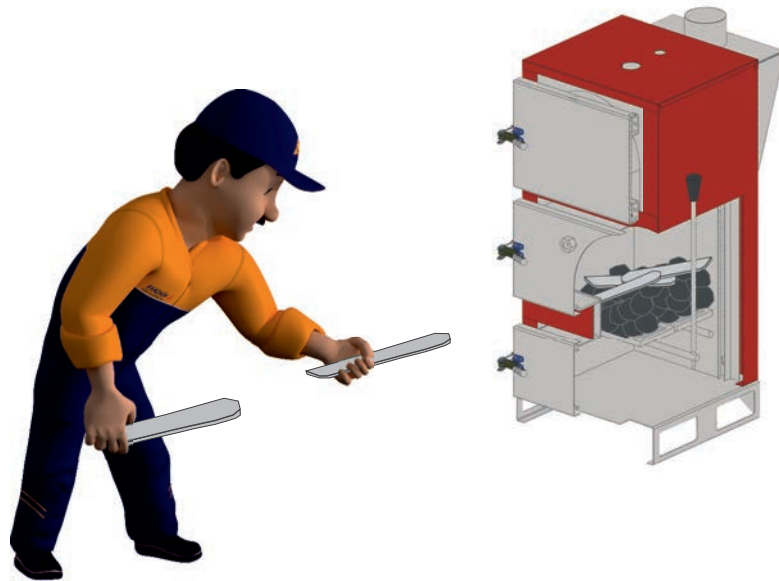
Figure 13: place wood pieces on fuel.
