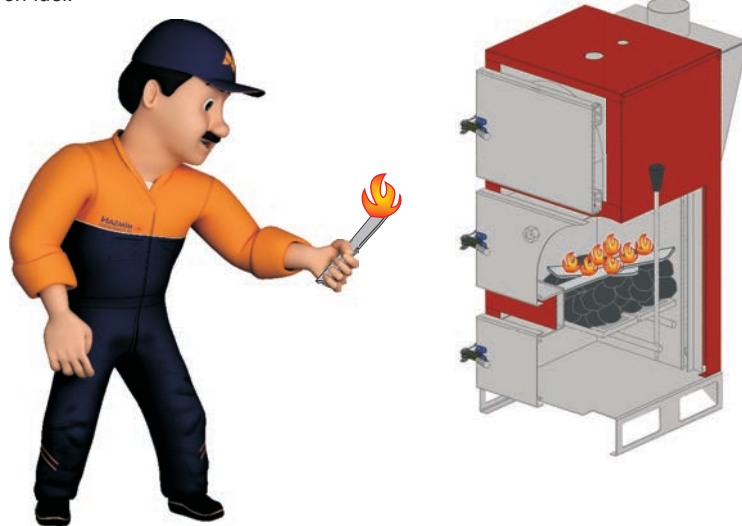
Figure 14: Ignite the wood pieces. Run the fan in a low cycle when the wood chips are well ignited.
