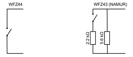
A cable break or short-circuit is detected when using the add-on module with NAMUR circuit; the receiving unit recognizes and registers it.
